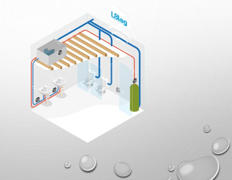
Temperature sensors are strategically installed at prechosen locations. This takes minutes, is not disruptive and the equipment will not be seen by day to day users.
